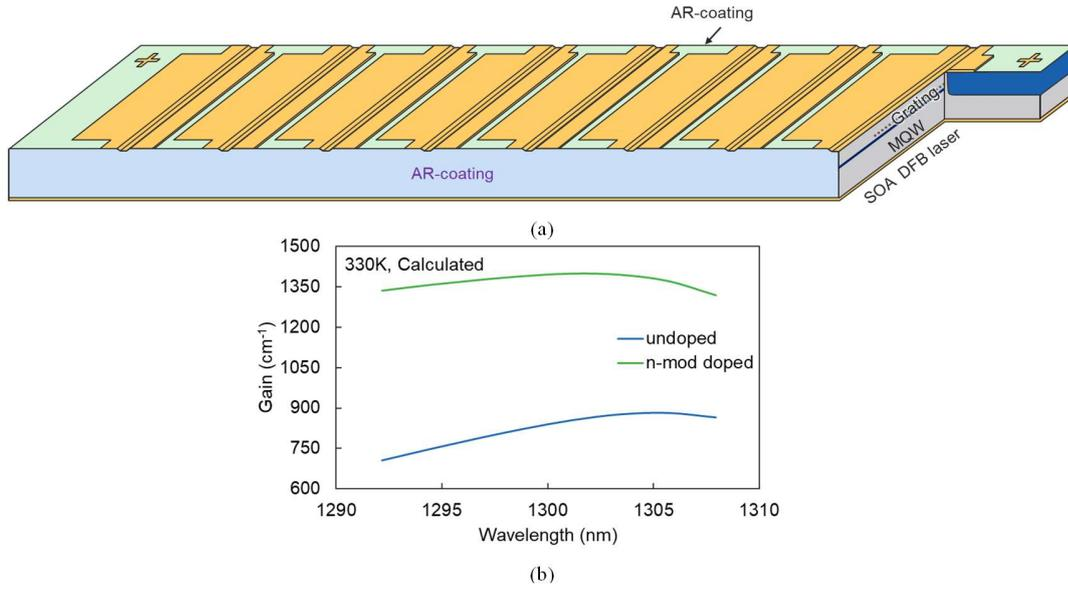
Fig. 1 (a) Schematic view of 8-channel CW-DFB laser array, (b) gain distribution comparison of undoped and n-modulation doped structure at the same carrier density.
