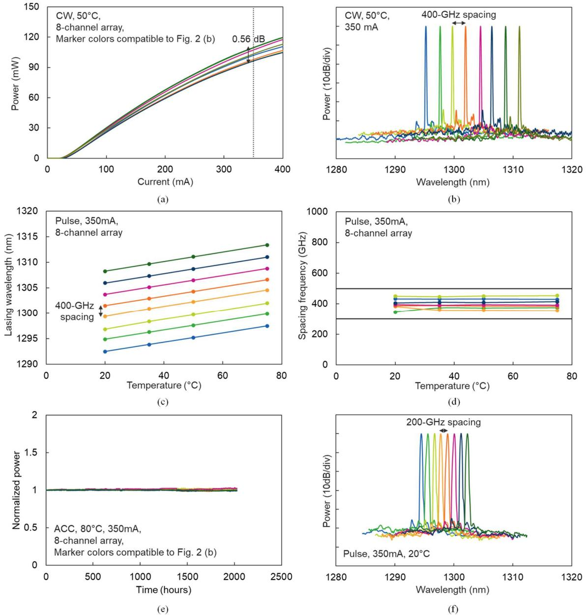
Figure 2 (a) I-L characteristic, (b) wavelength spectra, (c) temperature dependence of lasing wavelength, (d) spacing frequency, (e) power evolution at aging test of 400-GHz spacing laser array, and (f) wavelength spectra of 200-GHz spacing laser array.
