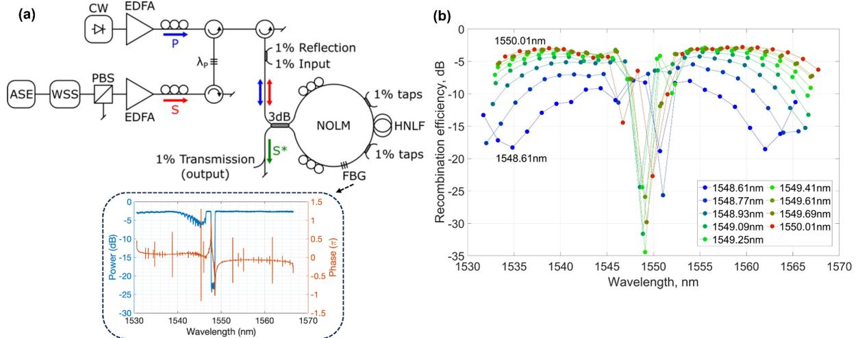
Fig. 1. (a) Schematic diagram of the experimental setup of the waveband-shift-free OPC. The inset shows the power and phase responses of the FBG. (b) Recombination efficiency of the signal conjugates at the NOLM output port as the pump wavelength is adjusted from 1548.6 nm to 1550 nm (see the legend for the exact values).
