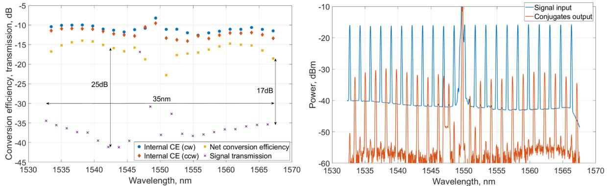
Fig. 2. (a) Overall optimized internal (clockwise – blue, counter-clockwise – red) and net (yellow) conversion efficiencies and signal transmission (purple). (b) Optical power spectra at the NOLM input and output.
