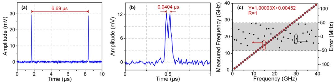
Fig. 4. Frequency measurement results for (a) a single-tone signal, (b) a two-tone signal, and (c) a tunable signal from 1 GHz to 39 GHz.
