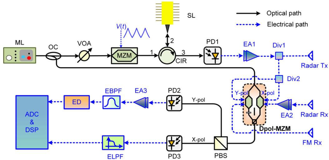
Fig. 1. Schematic diagram of the proposed integrated system for radar detection and frequency measurement.
