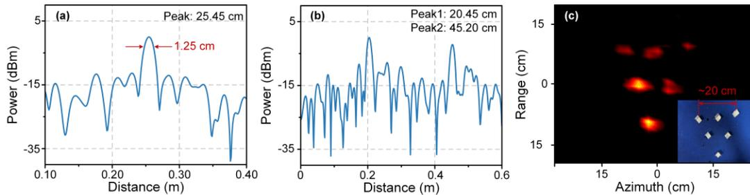
Fig. 3. Radar detection results for (a) a single target and (b) two targets; and (c) ISAR imaging.
