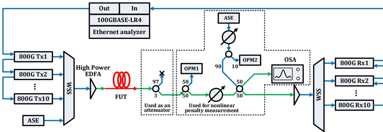
Fig. 2 Setup of real-time 40×800Gb/s DP-64QAM-PCS transmission over a fiber link.
