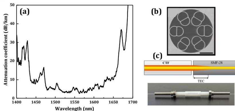
Fig. 1 (a) Measured loss spectrum and (b) cross-section of CTF. (c) Schematic mode evolution and (d) photograph of a CTF-SMF interconnection.
