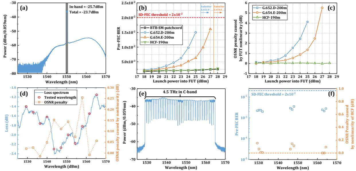
Fig. 3 (a) Measured output spectrum of EDFA. (b) Measured pre-FEC BERs and (c) derived OSNR penalties caused by nonlinearity of FUTs under different launch powers. (d) OSNR penalties measured at different wavelengths. (e) Output spectrum of  $40 \times 800$ -Gb/s DP-64QAM-PCS at receiver end. (f) Measured pre-FEC BERs and OSNR penalties of 10 different 800G channels.
