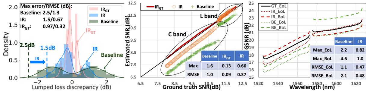
Fig. 3. (a) Lumped loss estimation in scenario 1 (3-span single OMS); (b) SNR estimation after 10 OMSes in scenario 2 (10 OMSes with 3 spans); (c) GSNR estimation with aging in scenario 3 (aging).
