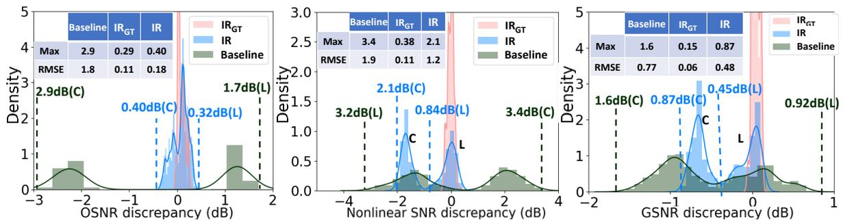
Fig. 2. (a) OSNR, (b) Nonlinear SNR, (c) GSNR estimation in scenario 1 (3-span single OMS).
