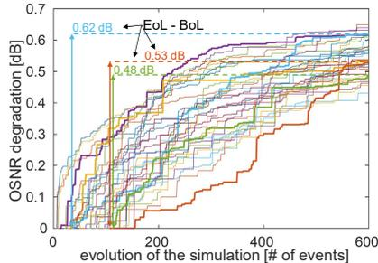
Fig2. Degradation of OSNR of a subset of lightpaths from BoL to the EoL.
