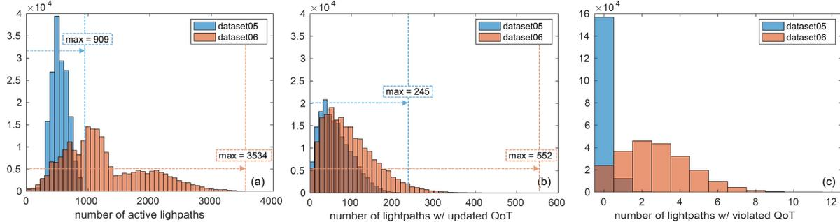
Fig1. Histograms of number of (a) active lightpaths, (b) lightpaths with updated QoT, and (c) lightpaths with violated QoT. The figures show samples of dataset05 and dataset06.
