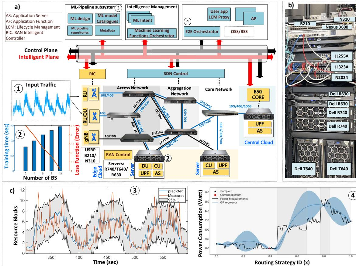
Fig. 1a) Network configuration, b) Experimentation infrastructure, c) ML pipeline for energy minimization: 1) Input traffic flows, 2) Optimal Placement of ML functions, 3) GPR model estimating RBs in RAN, 4) E2E Energy-aware optimization: The Bayesian solver identifies optimal routing strategy (red dot) minimizing power consumption. Results extracted for incoming traffic 150Mbps.
