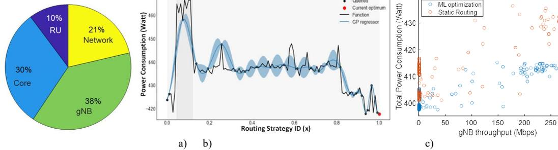
Fig. 2. a) Power consumption per domain, b) Energy-aware optimization using Bayesian techniques: Example for traffic/gNB 300Mbps, c) Total power consumption as a function of traffic/gNB for the static and dynamic routing using ML optimization.
