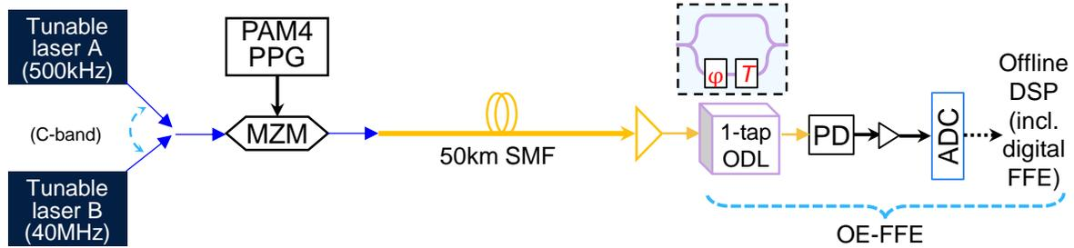
Fig. 1. Experimental setup of C-band OE-FFE-based 100Gb/s PAM4 over 50km SMF using laser with different frequency and linewidth. The inset shows the structure of the 1-tap ODL.  $\phi$ : phase shift.  $T$ : optical delay.
