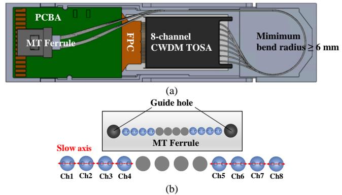
Fig. 2 Illustration for a QSFP ELS adopted with a blind optical connector. (a) Top view of the structure in the housing. (b) Optical interface.
