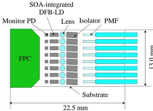
Fig. 1 Schematic illustration for the 8-channel CWDM TOSA structure.
