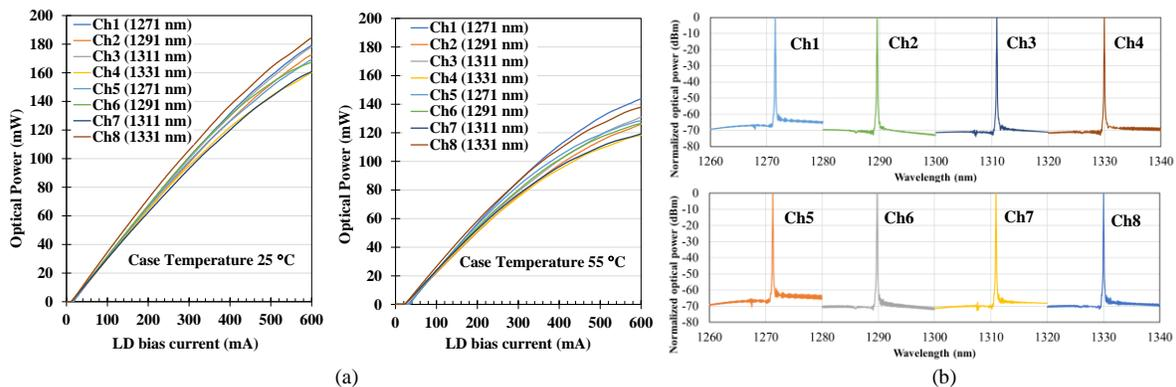
Fig. 4 Fiber-coupled power as a function of LD bias current and optical spectra. (a) L-I curves at the case temperature of 25 °C and 55 °C. (b) Optical spectra at the case temperature of 25 °C.
