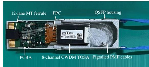
Fig. 3 Photograph of the 8-channel CWDM TOSA built in a QSFP housing with a PCBA. The PMF cables are turned with a bend radius of 7.5 mm to draw back to the card edge.
