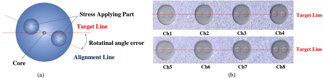
Fig. 5 Schematic illustration for the definition of rotational angle error and photographs of the PMF end face. (a) Definition of rotational angle error. (b) Photographs of the PMF end face.
