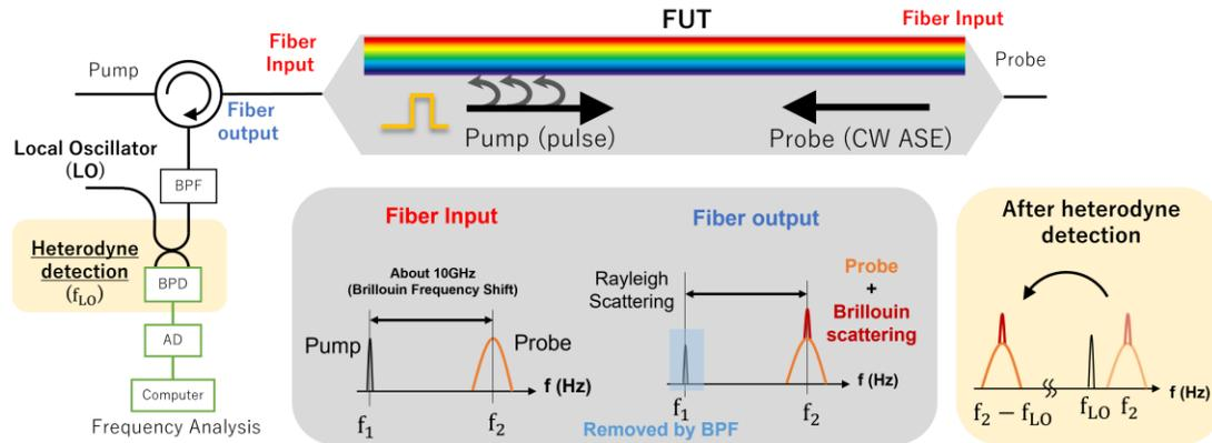
Fig. 1. Principle of ASE based BOTDA
