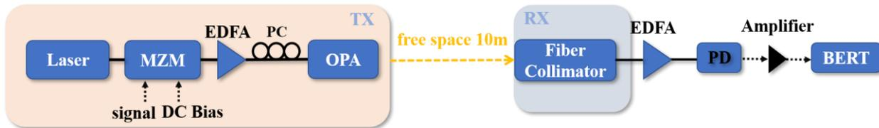
Fig. 2. Experimental setup of an OPA-embedded optical wireless communication system for the PAM4 optical signal transmission over 10 m.
