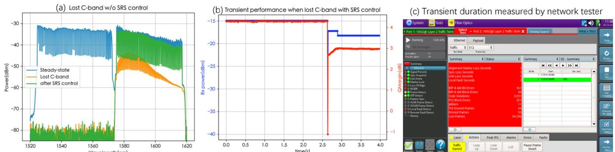
Fig. 5 (a) Spectra when lost C-band, (b) transient performance with SRS control, (c) network tester showing less than 2ms service disruption
