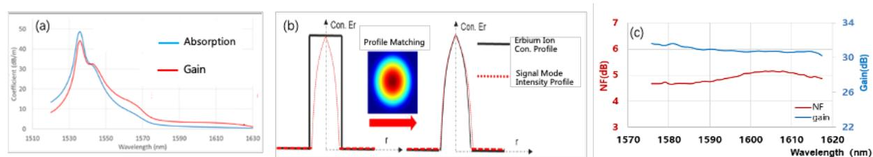
Fig. 2 L-100 EDFA: (a) Absorption and gain coefficients; (b) Erbium ion and signal mode intensity profile; (c) NF and gain.
