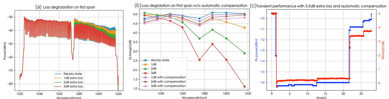
Fig. 3. Span loss degradation on first span: (a) Spectra, (b) Q-margin w/o compensation, (c) transient performance at longest L-band wavelength
