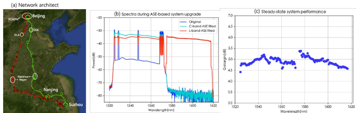
Fig. 1 (a) System architect of the deployed network; (b) spectra during L-band upgrade; (c) steady state Q-margin of all channels.
