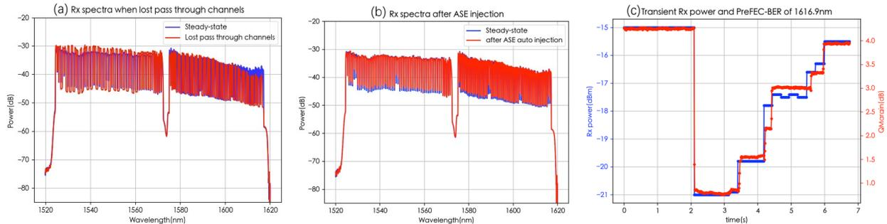
Fig. 4 ASE automatic injection: (a) spectra when loss half channels, (b) spectra after ASE injection, (c) transient performance at 1616.9nm.
