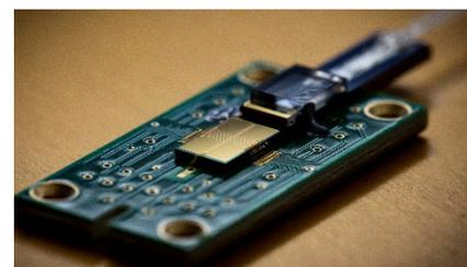
Figure 4. Quantum ion trap PIC assembled with a PCB and fiber optic input by ETH Zurich [9]. Reprinted with permission.
