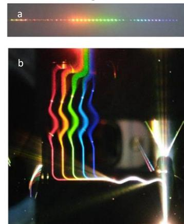
Figure 2. Cascaded AWGs for visible spectrum identification. (a) shows the end facet view, and (b) shows the top view.
