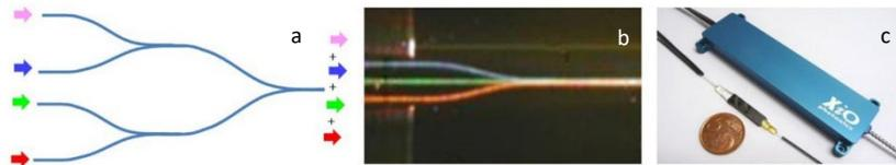
Figure 1. An integrated laser beam combiner. (a) shows a waveguide schematic illustrating its function. (b) shows the PIC in action. (c) shows the complete packaged module.
