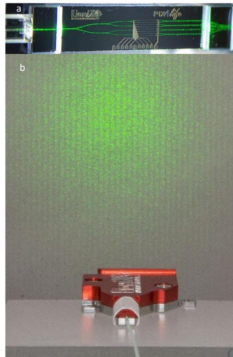
Figure 3. Variable optical attenuators in action. (a) shows the PIC with splitters and MZIs. (b) shows the packaged module projecting the light onto a screen.
