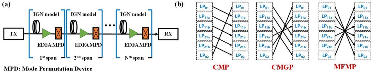
Fig. 1. (a) FMF transmission systems with mode permutation, evaluated using the IGN model, (b) mode permutation strategies (CMP: cyclic mode permutation [7], CMGP: cyclic mode-group permutation [8], MFMP: mirror-flipped mode permutation [9]). The CMP and CMGP schemes [7,8] take 6 and 4 spans as one period of permutation to realize the cyclic shift of all spatial modes, respectively, and the MFMP scheme [9] takes 2 spans as one period of permutation to realize more frequently modes exchanging.
