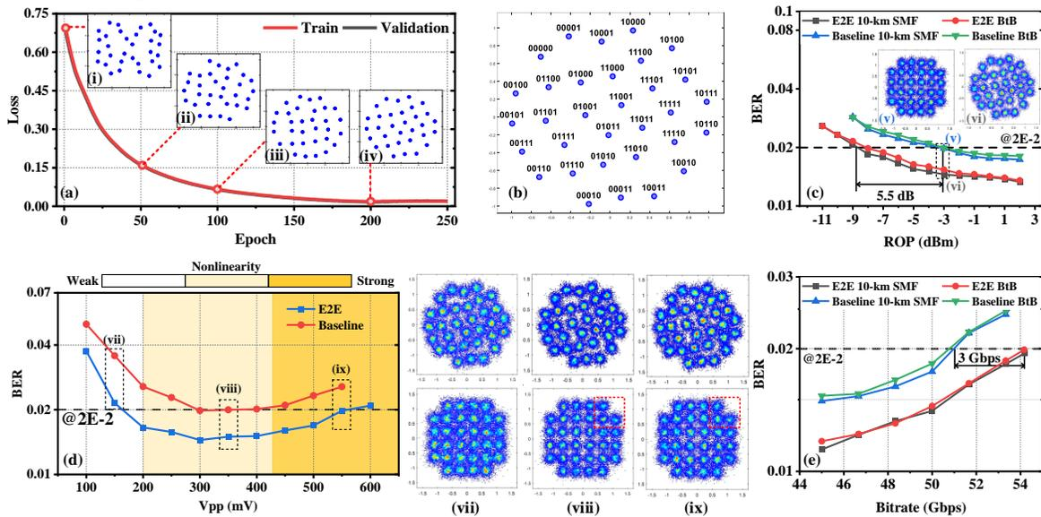
Fig. 3 (a) The learning curve of the autoencoder network; (b) The learned bits-to-symbol mapping rule; (c) The BER of the fiber-THz integrated system with different (c) ROP, (d)  $V_{pp}$ , and (e) Bitrate.
