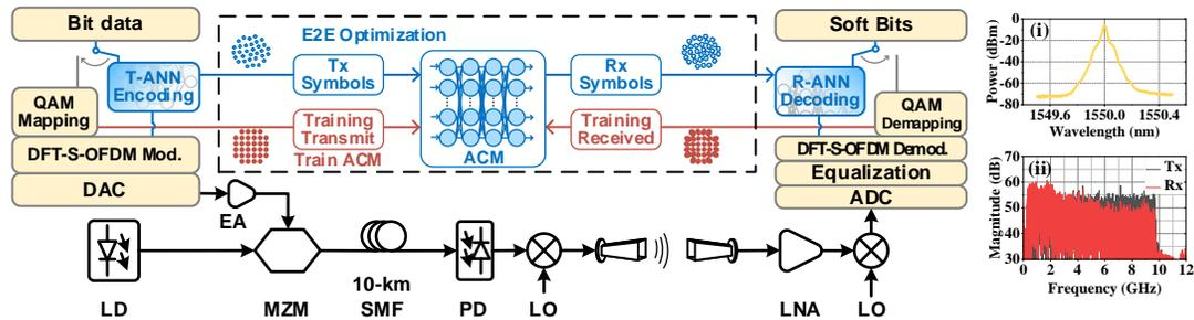
Fig. 2 Experimental setup of the fiber-THz integrated E2E optimized DFT-S-OFDM communication system, (i) is the optical spectrum of the received signal at the photodiode (PD), (ii) is the spectrum of the transmitted (Tx) and received (Rx) signal.
