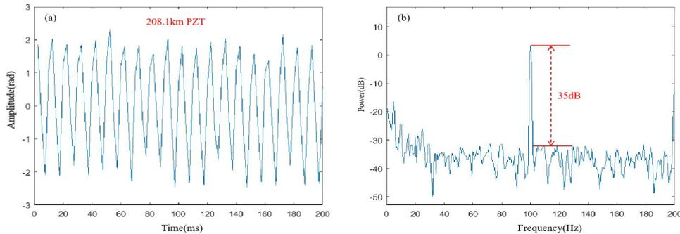
Figure.3. (a) Demodulated 100Hz phase signal at 208.1km PZT; (b) The spectra of the demodulated phase signal.
