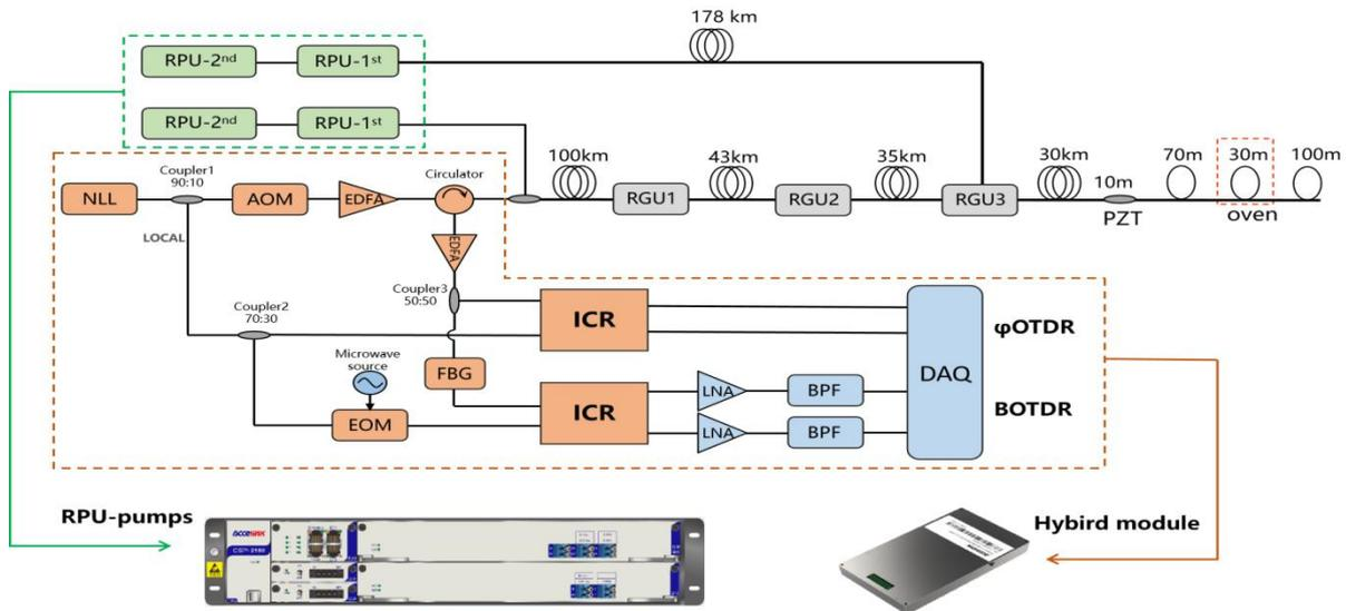
Fig.1. Experimental setup. NLL: narrow linewidth laser; AOM: acousto-optic modulator; EDFA: Erbium Doped Fiber Amplifier; ICR: Integrated coherent receiver; EOM: electro-optic modulator; FBG: Fiber Bragg Grating; LNA: low noise amplifier; BPF: band-pass filter; DAQ: data acquisition card; RPU: remote pumping unit; RGU: remote gain unit; PZT: piezoelectric transducer;
