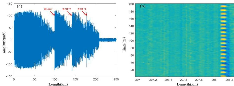
Fig. 2. (a) Time domain traces of Rayleigh trace; (b) 3D map of the distribution of the vibration.
