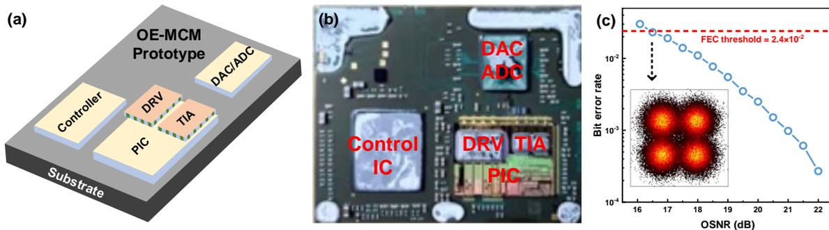
Fig. 2 (a) Schematic and (b) photo of the single-carrier 400G DP-QPSK transceiver prototype; (c) B2B BER curve versus OSNR.
