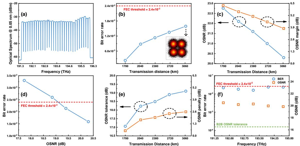
Fig. 3 (a) Measured B2B optical spectrum with a wavelength resolution of 0.05 nm; (b) BER curve versus transmission distance (the inset is the recovered QPSK constellation diagram); (c) curves of OSNR and OSNR margin versus transmission distance; (d) BER curve at the transmission reach versus OSNR; (e) curves of OSNR tolerance and OSNR penalty versus transmission distance; (f) the curves of BER and OSNR at the transmission reach versus five WDM channels under test.
