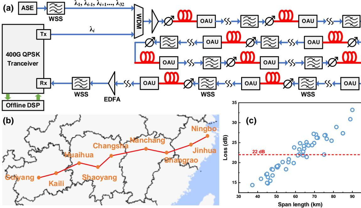
Fig. 1 (a) Schematic of the single-carrier 400G DP-QPSK transmission over 3075-km G.652.D fiber link with a configuration of emulating (b) the field deployment from Ningbo City to Guiyang City in China (OAU: optical amplifier unit which consists of BDRA and EDFA for spans with loss larger 22 dB, and is just EDFA for else spans); (c) scatter diagram of total loss for 49 spans versus the corresponding field-deployed length.
