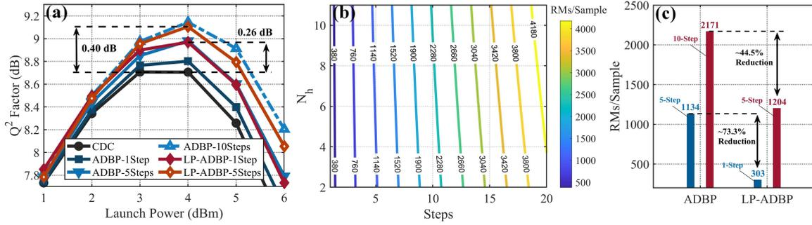
Fig. 3. (a) The performance of different algorithms. (b) The complexity of LP-ADBP measured by real multiplications per sample (RMs/Sample) with respect to  $N_h$  and steps. (c) The complexity comparison between 5-Step ADBP, 10-Step ADBP, 1-Step LP-ADBP, and 5-Step LP-ADBP.
