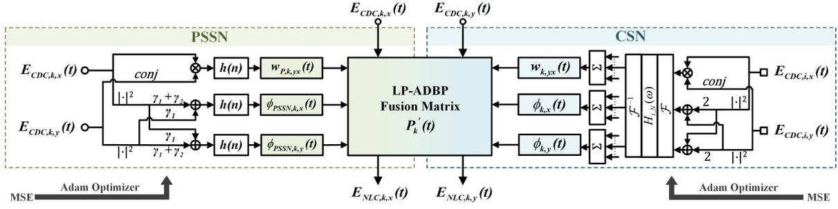
Fig. 1. Block diagram of one NLC step in the proposed LP-ADBP.
