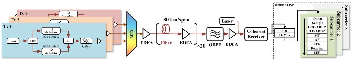
Fig. 2. Block diagram of the 9-channel 8-subcarrier SCM simulation system.
