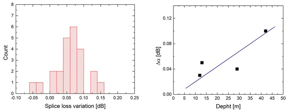
Fig.2: Histogram of the variation of losses in splice boxes (left) and variation of the losses with depth (right)
