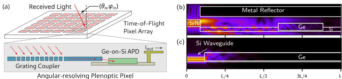
Fig. 1: (a) Operating principle of a plenoptic ToF sensor. A grating coupler acts as an angular-selective filter to separate light by the angle of incidence. An array of such pixels can be used to create a small form factor, short-range LiDAR sensor. (b-c) Comparison of (b) edge-coupling with minimum SiN-Ge space and (c) waveguide-coupling coupling efficiency. In the edge-coupling case, only  $\sim 30\%$  of the light is absorbed in the Ge absorption region vs.  $>95\%$  for waveguide-coupling.
