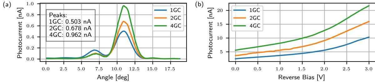
Fig. 3: Experimental results demonstrating photocurrent scaling for 1, 2 and 4 grating couplers. (a) Photodetector response vs. incident angle, demonstrating the angular selectivity of the arrays. (b) Photocurrent vs. reverse bias voltage at the peak coupling angle.  $V_R$  for these devices was restricted to 3V due to reliability limitations.
