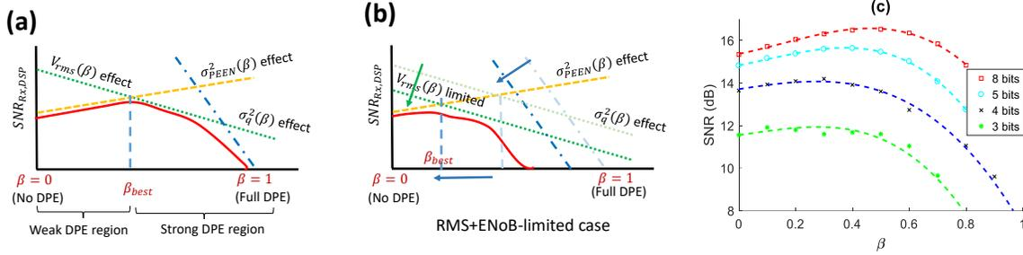
Fig. 1. (a) The three main contributions to determine SNR under Tx constraints (b) RMS and ENoB-limited scenario (c) Simulated impact of quantization effect in the presence of tight filtering on SNR versus  $\beta$ , EDFA gain = 22dB, noise loading at receiver
