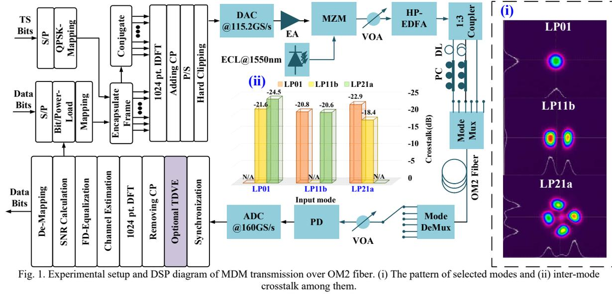
Fig. 1. Experimental setup and DSP diagram of MDM transmission over OM2 fiber. (i) The pattern of selected modes and (ii) inter-mode crosstalk among them.
