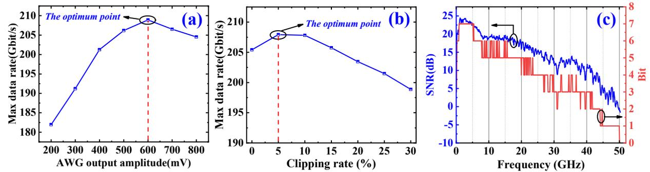
Fig. 2. (a) Max transmission data rate vs. AWG output amplitude, (b) Max transmission data rate vs. clipping rate and (c) Channel response and bit allocation for LP01 mode channel.
