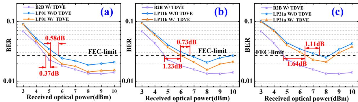
Fig. 3. BER vs. ROP with/ without TDVE for (a) LP01, (b) LP11b and (c) LP21a mode.
