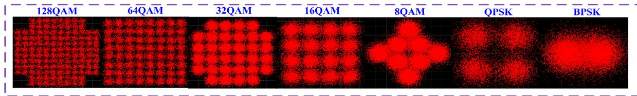
Fig. 4. Received bit-loading DMT signal constellations of LP21a mode with ROP of 7dBm
