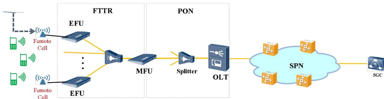
Fig.3 Schematic setup of the field trial of FTTR based 5G small cell backhaul
