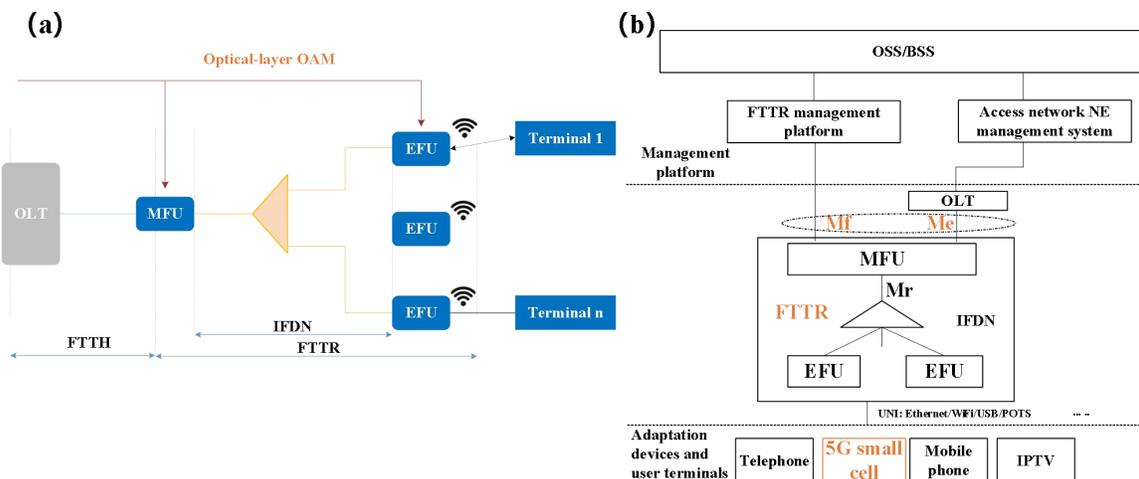
Fig.1 (a) Network location of FTTR system; (b) The proposed native management architecture of FTTR system
