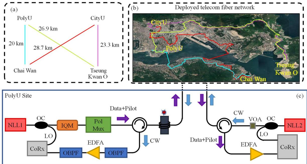
Fig. 1. (a) Routine of the deployed fiber link (b) Map of the deployed fiber network and (c) Experimental setup of the proposed integrated sensing and communication system.
