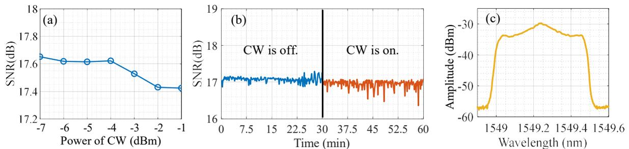
Fig. 2. (a) Measured SNRs of the 16 QAM signal when the power of CW is increased from -7 dBm to -1dBm; (b) Long-term SNR as the counter-propagated CW light is switched on or off; (c) Optical spectrum of the 16 QAM signal at the receiver when CW is on.
