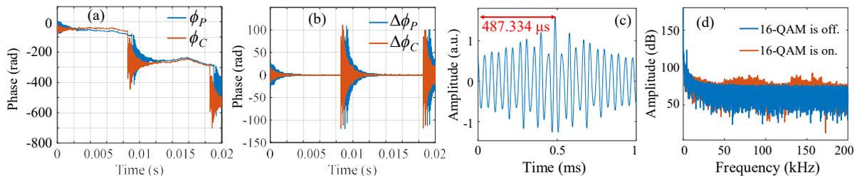
Fig. 3(a) Extracted phase profiles of CW tone  $\phi_C(t)$  and pilot tone  $\phi_P(t)$ ; (b) phase profiles  $\Delta\phi_C(t)$  and  $\Delta\phi_P(t)$  after high-pass filtering; (c) cross-correlation between  $\Delta\phi_C(t)$  and  $\Delta\phi_P(t)$  and (d) effect of the 16-QAM communication signal on the spectra of  $\phi_C(t)$ .
