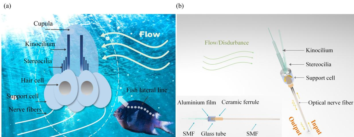
Fig. 1. (a) Schematic diagram of a fish's neuromast. (b) The structure of optical fiber artificial neuromast.
