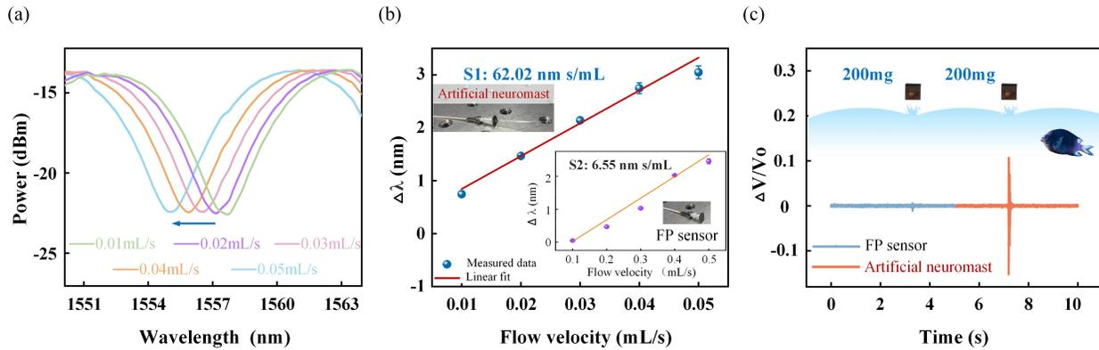
Fig. 3. (a) Evolution of reflection spectra of the artificial neuromast as the velocity increased. (b) The dip wavelength versus flow velocity and sensitivity comparison of artificial neuromast and usual FP sensor. (c) The detection comparison of water disturbance.
