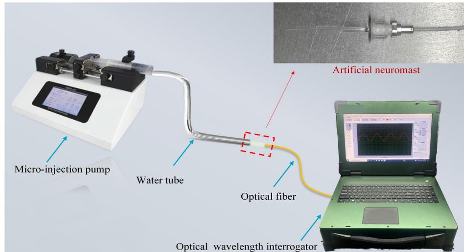
Fig. 2. The experimental setup of the water flow monitoring system. The inset shows the photograph of the artificial neuromast.
