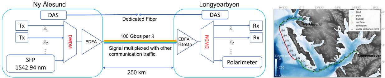
Fig. 1. Schematic of the field test setup and the map of Svalbard where the cable is placed
