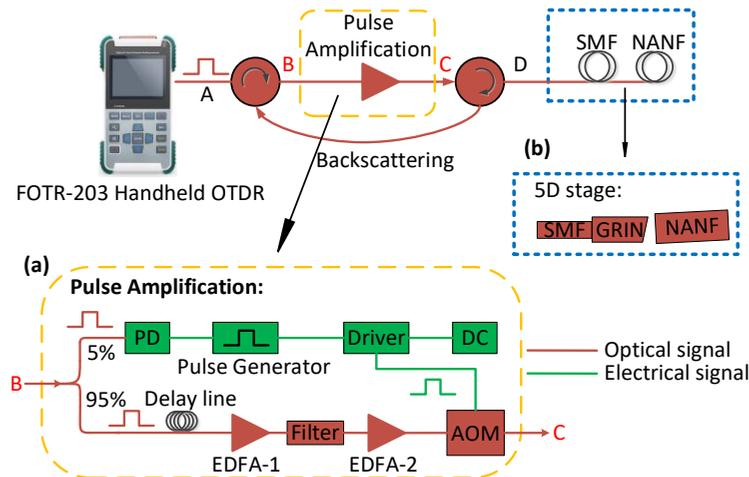
Fig. 1. Experimental setup showing the detail of the implemented Pulse Amplification unit (a) and detail of SMF-NANF light coupling (b). PD: photodetector, AOM: acousto-optic modulator.
