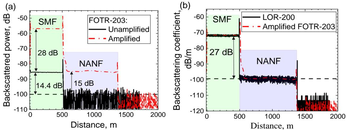
Fig. 2. OTDR traces using 10 ns pulses for a FUT consisting of 509-m SMF and 885-m NANF measured with the FOTR-203 both without and with the Pulse Amplification unit (a). For comparison, backscattering coefficients obtained from measurements with the Pulse Amplified FOTR-203 and with a high end LOR-200 OTDR without Amplification unit (upgraded version of that used in [5] are shown in (b).
