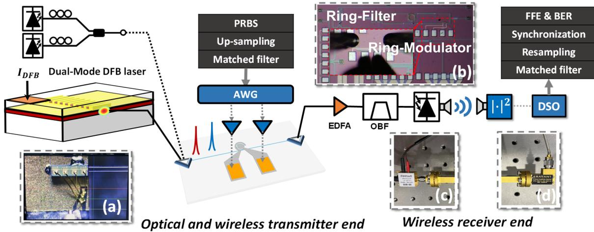
Fig. 1. Experimental setup for a W-band IM-DD wireless communication system. (a) On-chip dual-mode DFB laser. (b) Silicon photonic integrated circuit (PIC) containing microring modulator and filter. (c) High-speed photodetector with W-band transmitting antenna. (d) Envelope detector with W-band receiving antenna.
