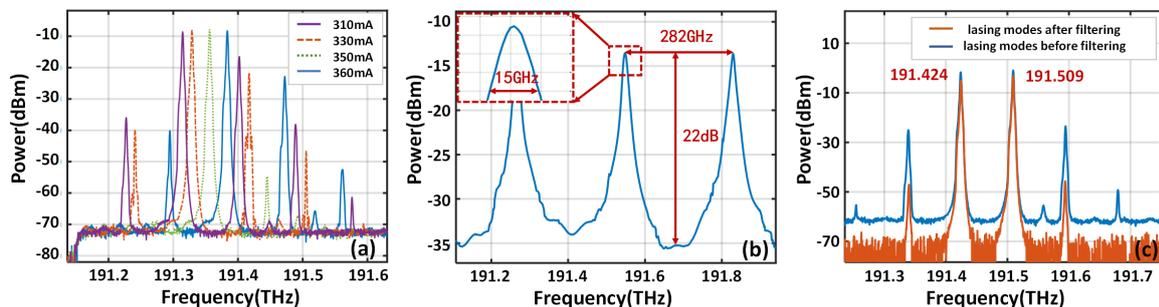
Fig. 2. (a) dual-mode and single-mode of DSB at different input currents. (b) transmission spectral line of on-chip ring filter. (c) modulated optical source and reference source before and after filtering.
