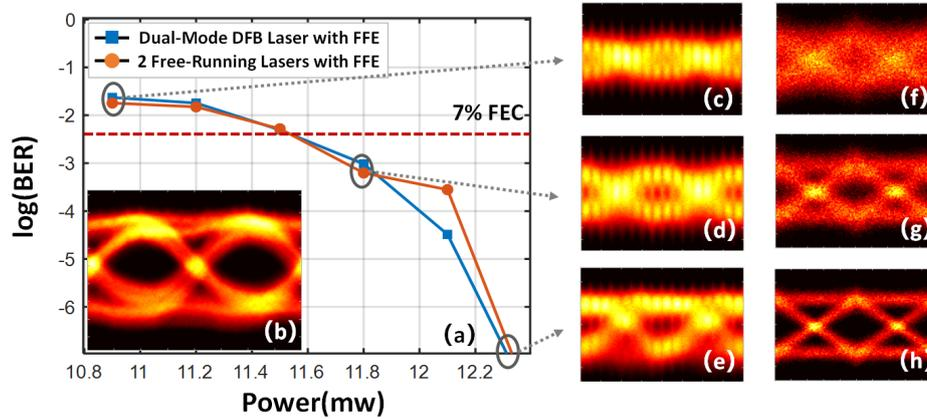
Fig. 3. (a) BER versus input optical power. (b) eye diagram before wireless transmission. (c-e) eye diagrams without processing. (f-h) eye diagrams with FFE equalizing.
