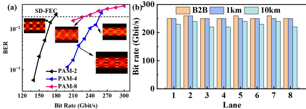
Fig. 3. (a) B2B BERs with respect to different data rates for PAM2, PAM4 and PAM8 signals of a single lane. (c) The highest PAM4 bit rates of 8 lanes with BERs below the SD-FEC threshold for B2B, 1 km and 10 km SMF transmissions.
