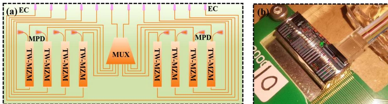
Fig. 1. (a) A floorplan of the 1×8 all-silicon LAN WDM transmitter. EC, edge coupler; MPD, monitoring photodetector; TW-MZM, traveling wave Mach-Zehnder modulator; MUX, multiplexer. (b) Micrograph of the all-silicon transmitter chip packaged on the evaluation printed circuit board (PCB).
