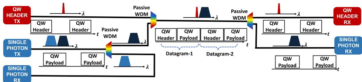
Fig. 1. A schematic of the point-to-point WDM QW datagram transmission
