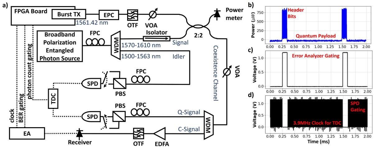
Fig. 2. a) Schematic of the experimental setup. b) Optical output of the burst TX. c) Electrical signal from FPGA board to gate EA. d) Electrical signal from FPGA to gate SPD and clock TDC.
