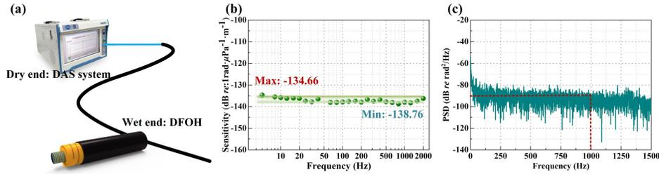
Fig.1 (a) The system based on  $\varphi$ -OTDR and DFOH with BEOF; (b) The calibrated frequency response from 5Hz to 2kHz; (c) The noise PSD of the system.
