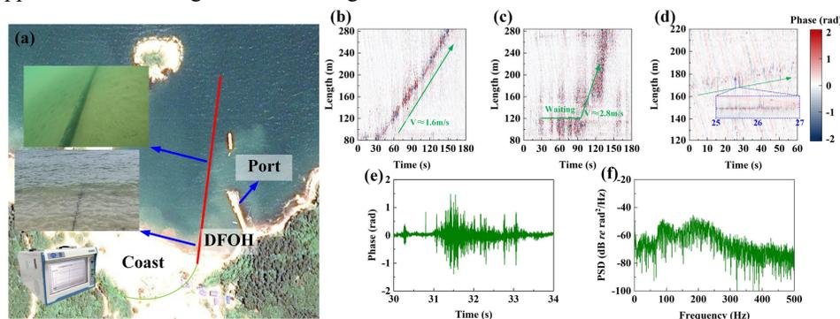
Fig.3 (a) The system setup of the sea trial; The space-time distribution of the (b) small boat, (c) assault boat, (d) and underwater frogman. (e) The time domain waveform, (f) and PSD of the frogman signal.
