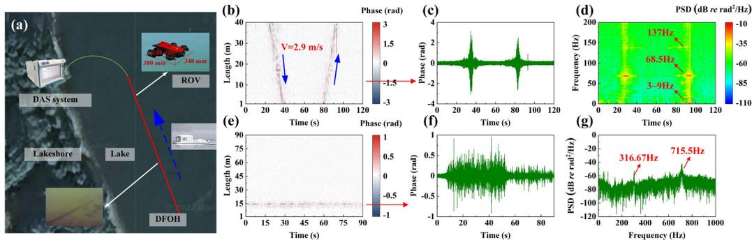
Fig.2 (a) The system setup of the lake trial; (b) The space-time distribution, (c) time domain waveform, (d) and time-frequency distribution of the assault boat in the lake trial; (e) The space-time distribution, (f) time domain waveform, (g) and PSD of the ROV signal.
