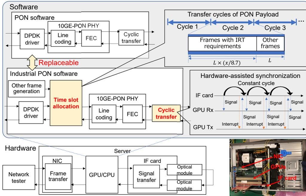
Fig. 2. Proposed PHY implementation of PON and industrial PON on a common server.
