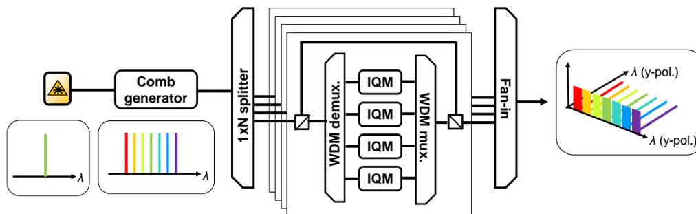
Fig. 1: Conceptual image of an uncooled SDM/WDM self-homodyne transmitter using a single laser.
