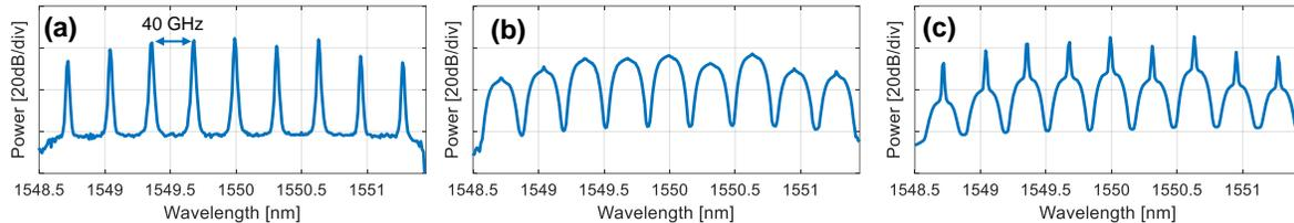
**Fig. 3:** Optical spectra of (a) the frequency comb, (b) IQ-modulated signals, and (c) polarization-multiplexed signals.
