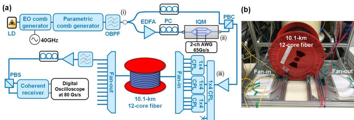
Fig. 2: (a) Experimental setup and (b) external appearance of the 12-core fiber.
