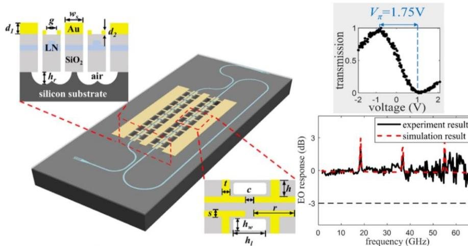
Fig. 2. A ring-assisted TFLN-based MZM feature high Q-factor and wide bandwidth [15].
