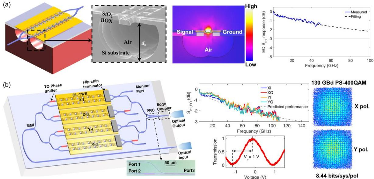
Fig. 1. (a) High-performance MZM based on LN-on-Silicon platform and silicon removal technology [12]. (b) Dual polarization IQ modulator based on LN-on-quartz platform for Tb/s transmission [13].
