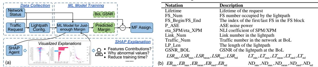
Fig. 2. (a) The framework of the explainable machine learning-enabled just-enough margin configurations. (b) Notations of the input features.
