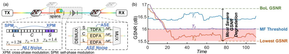
Fig. 1. (a) Different transmission effects in different bands; (b) Illustration of GSNR degradation and just-enough margin configuration.
