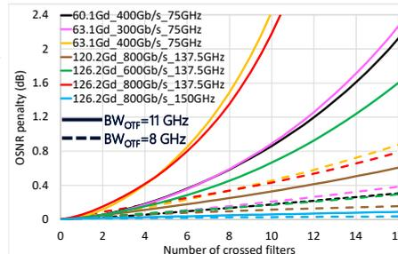
Fig.2: OSNR penalties across a suite of filters, w.r.t modulation & filter sharpness
