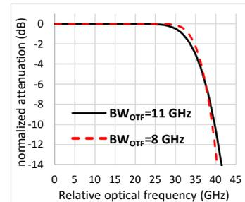
Fig.3: Comparison of lateral 75 GHz-wide WSS filter shapes
