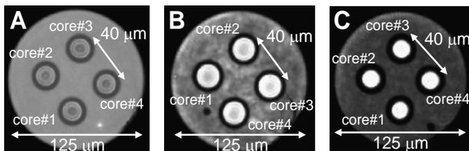
Fig. 1. Cross-sectional images of the TA-4CFs fabricated by vendors A, B, and C.
