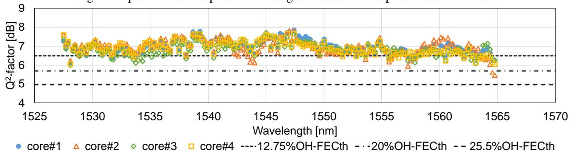
Fig. 8.  $Q^2$ -factors for all 4-SDM/188-WDM channels after 1,800-km transmission.
