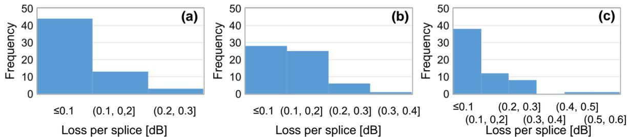
Fig. 6. Histograms of the losses per splice at 1550 nm in (a) Cable A, (b) Cable B, (c) Cable C.
