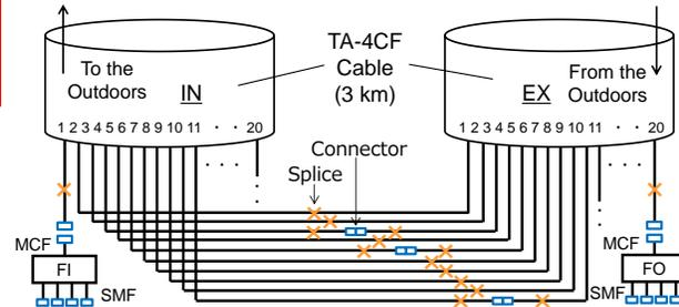
Fig. 5. 60-km TA-4CF configuration with splices and connectors.
