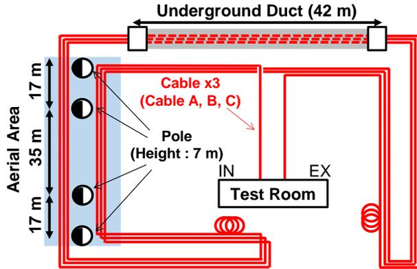
Fig. 3. Cable route of the installed TA-4CF cables.
