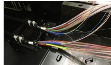
Fig. 2. A snapshot of the prototype MCF cable fabricated using these TA-4CFs.
