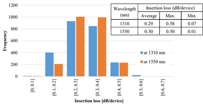
Fig. 3. ILs of the fanout devices (612 devices, 2448 channels).
