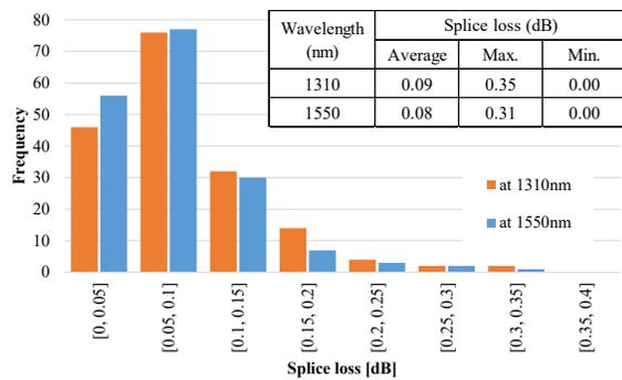
Fig. 2. Splice loss measurement result of 4c-MCF (44 connections, 176 cores).
