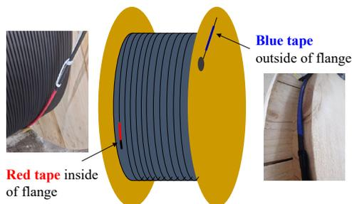
Fig. 7. MCF cable drum with polarity identifications.
