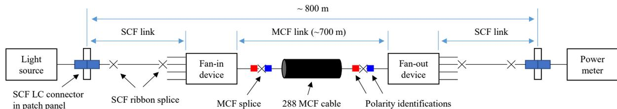
Fig. 4. Schematic of a field deployed, panel-to-panel MCF link with OLTS measurement setup.
