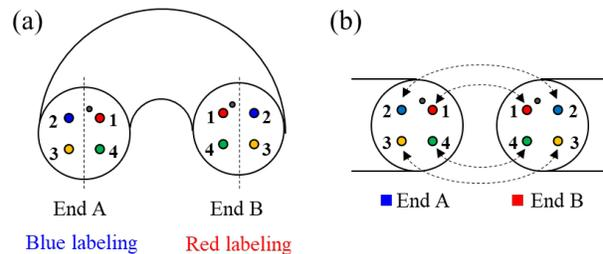
Fig. 6. (a) Definition of MCF polarity and labeling color. (b) Connected core numbers in MCF-to-MCF connection.
