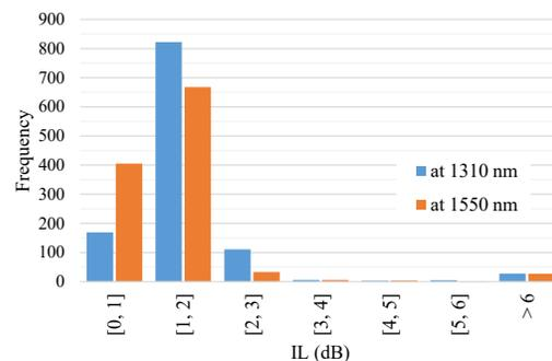
Fig. 8. OLTS result of the MCF link (1152 channels).
