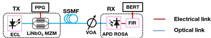
Fig. 1. Experimental setup
