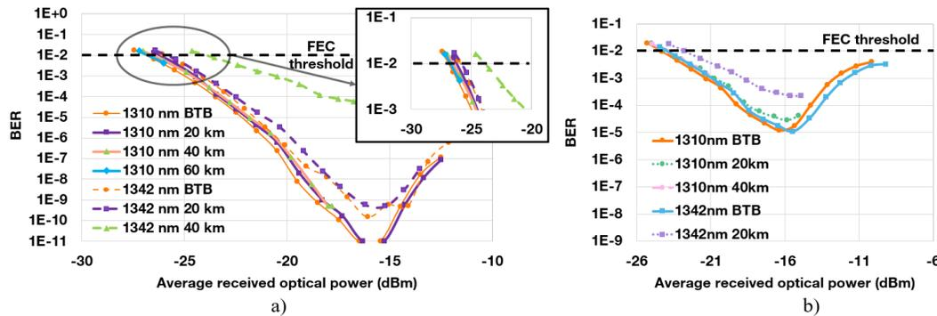
Fig. 4. (a) BER versus received optical power at 1310 nm and 1342 nm for 0, 20, 40 and 60 km. (b) BER versus received optical power at 1310 nm and 1342 nm in NRZ at 58.2 Gbit/s.
