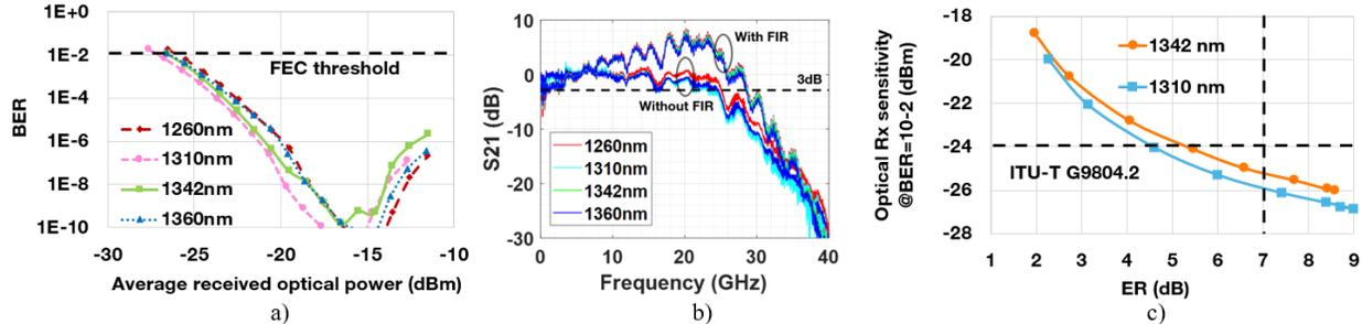
Fig. 2. a) BER versus average received optical power for 1260 nm, 1310 nm, 1342 nm and 1360 nm. b) Frequency response of the APD-ROSA with and without FIR filter. c) Receiver sensitivity at  $BER=10^{-2}$  as function of the extinction ratio for 1310 nm and 1342 nm.
