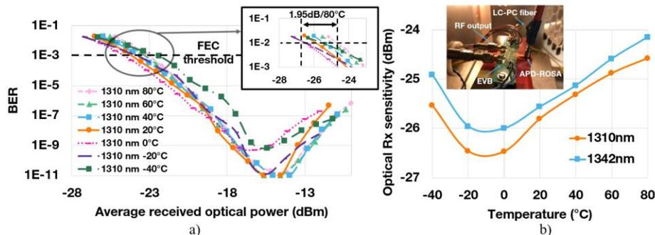
Fig. 3. (a)) BER as function of the average received optical power at 1310 nm for temperature from -40°C to 80°C. (b)) Receiver sensitivity at 1310 nm and 1342 nm for temperature from -40°C to 80°C
