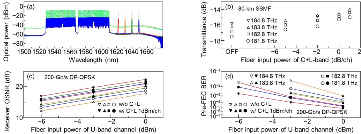
Fig.2. (a) optical spectra before (dotted) and after (solid) 80-km SSMF transmission, (b) transmission loss dependent on C+L-band channel power, (c) receiver OSNR for U-band channels, and (d) pre-FEC BER of U-band channel after 80-km SSMF transmission.
