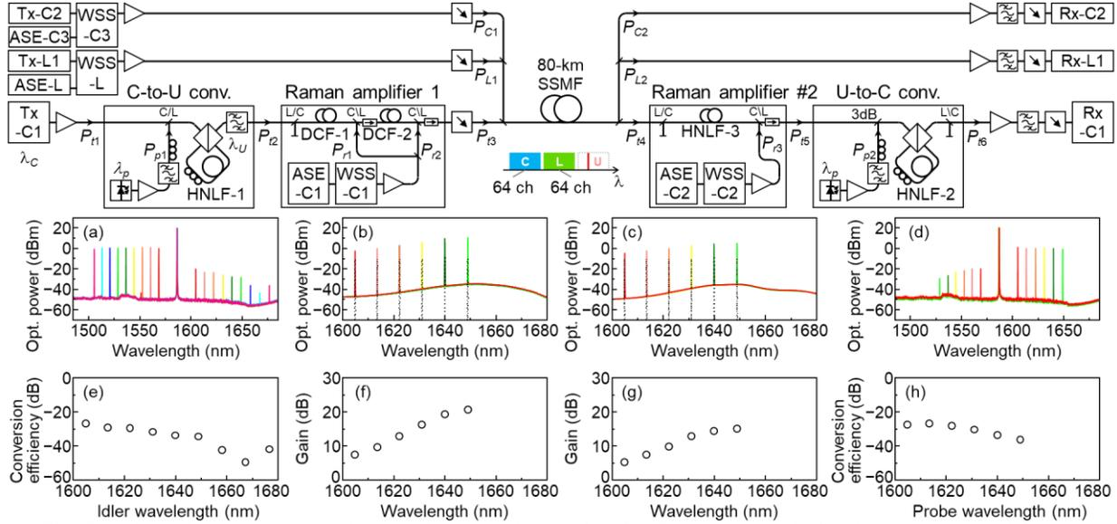
Fig. 1 Experimental setup, output optical spectra (0.1-nm resolution) of (a) C-to-U converter, (b) the first discrete Raman amplifier, (c) the second discrete Raman amplifier, and (d) U-to-C converter, conversion efficiency of (e) C-to-U converter and (h) U-to-C converter, and gain of (f) the first discrete Raman amplifier and (g) the second discrete Raman amplifier
