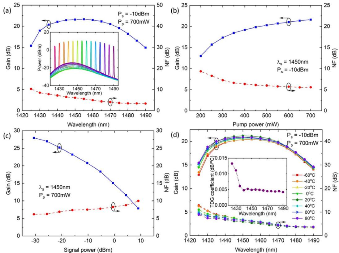
Fig. 2. (a) Gain and NF spectrum from 1425nm to 1490nm at RT for a -10dBm signal (the inset shows the signal and noise spectra from which the in-band OSNR is derived); (b) Gain and NF variation with pump power for a -10dBm signal at 1450nm; (c) Gain and NF variation with signal power at 1450nm; (d) Gain and NF spectra in the temperature range from -60°C to +80°C at intervals of 20°C for a -10dBm signal (the inset shows the calculated TDG coefficient spectrum from 1425-1490nm).
