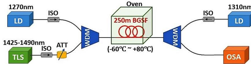
Fig. 1. Experimental setup of the E+S-band Bi-doped germanosilicate fiber amplifier.
