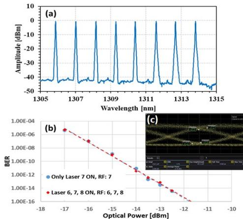
Fig.7: a) Tx output spectrum, b) BER performance at 32 Gb/s, c) Tx eye diagram at 64 Gb/s.
