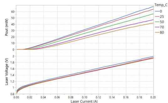
Fig. 1: DFB laser LI and IV from 0°C to 80°C.
