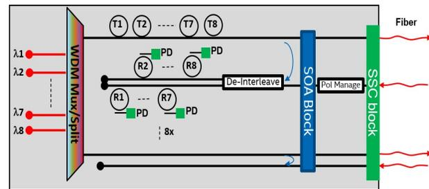
Fig.6: Block diagram of the 4 Tb/s OCI SiPIC architecture.
