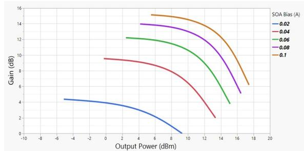
Fig. 2: SOA gain vs. output power at different bias currents.
