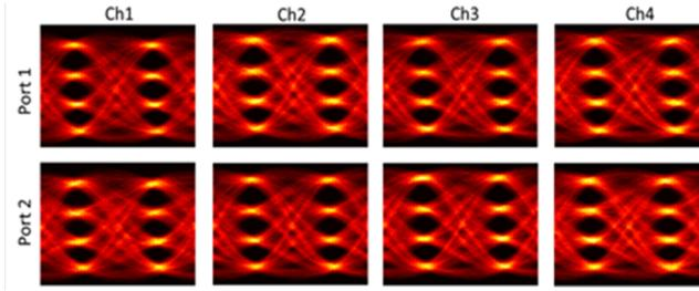
Fig. 5. Measured 106.25 Gb/s PAM4 Tx eye diagrams.
