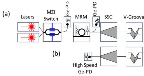
Fig. 4. SiPIC architecture for a) Tx and b) Rx channels.
