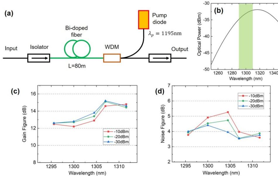
Fig. 1. (a) Schematic setup of the backward pumped BDFA, (b) measured ASE spectra of the BDFA, gain figure (c) and noise figure (d) of the BDFA at different input signal powers with a pump power of 500mW.
