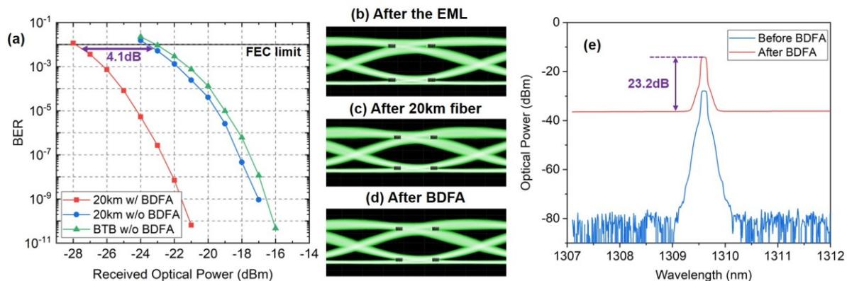
Fig. 3. (a) BER performances for 50Gb/s upstream signal, measured eye diagram of 50Gb/s NRZ signal (b) after the EML, (c) after 20km fiber transmission, (d) after BDFA amplification, (e) optical spectra of the small signal before and after amplification.
