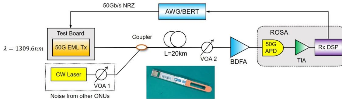
Fig. 2. Experimental setup for 50Gb/s upstream transmission with 20km SMF using a BDFA as preamplifier, (inset) photo of the commercial SFP56-DD type packed 50G EML transceiver.
