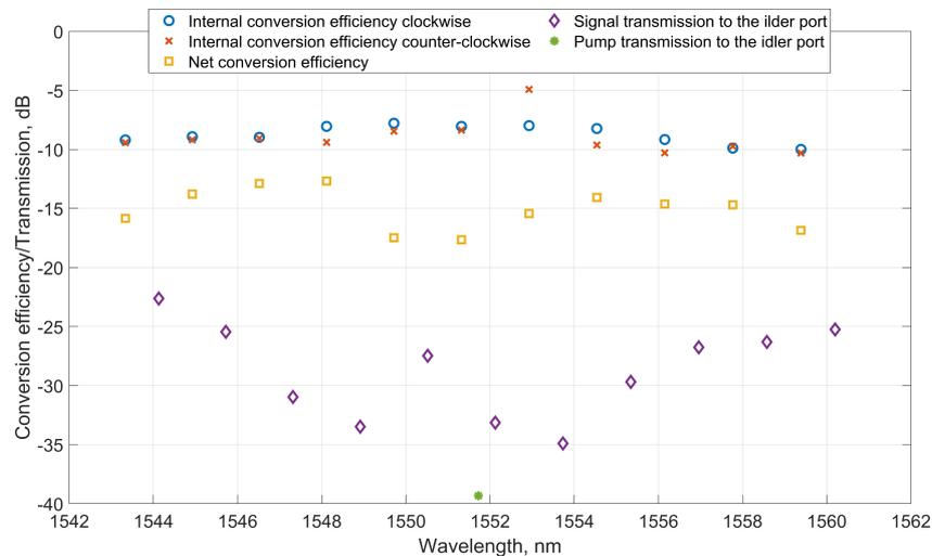
Fig. 3. Conversion efficiency in both directions inside the loop (blue circles and red crosses); Net conversion efficiency from the input to the output of the loop (yellow squares); and Signals and pump transmission from the input to the output of the loop (purple diamonds and the green star respectively).
