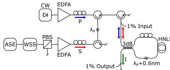
Fig. 1. Experimental setup of a waveband-shift free OPC in NOLM.
