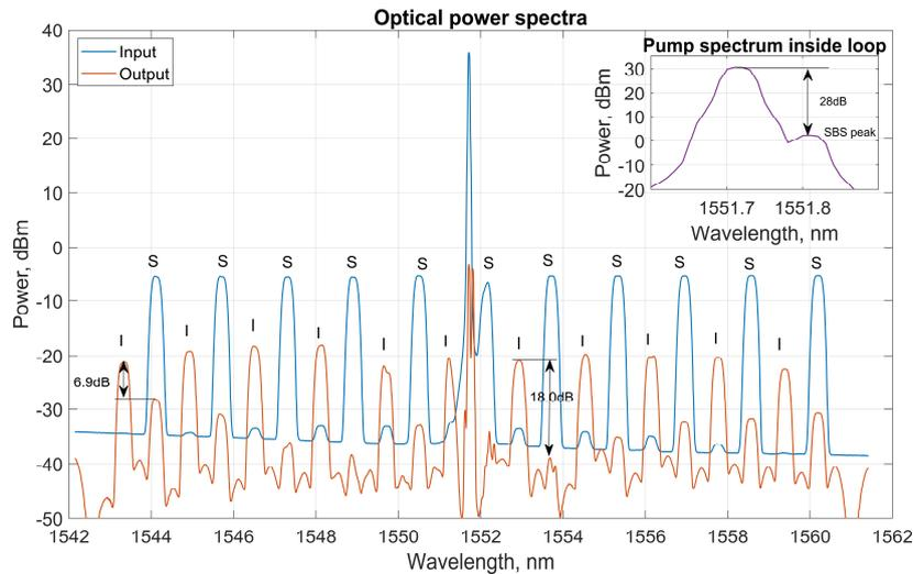
Fig. 2. Optical power spectra at the input and the output of the loop. Inset shows a zoomed pump spectrum measured inside the loop.
