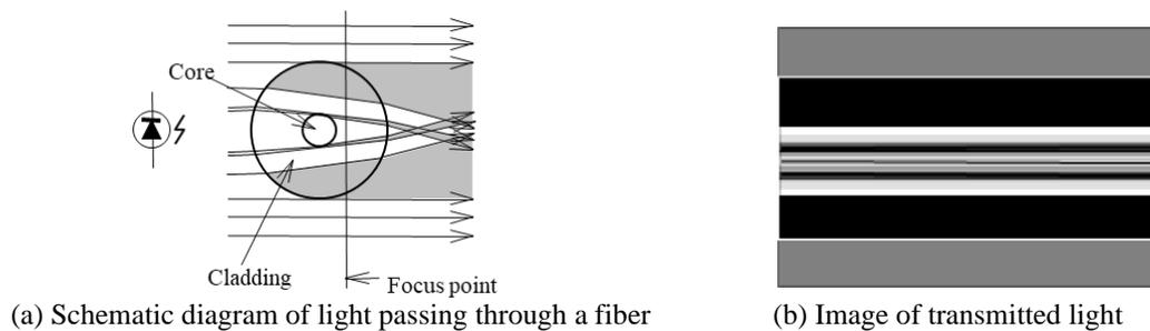
Fig. 3 Principle of core position measurement
