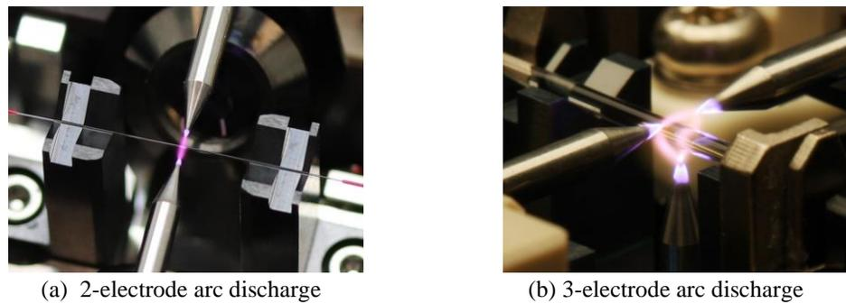
Fig. 1 Pictures of arc discharge systems
