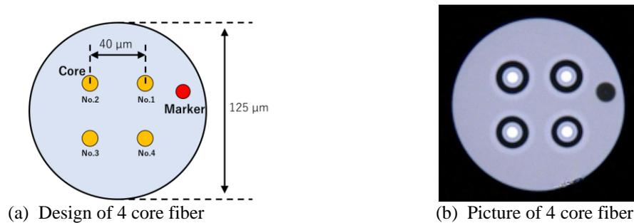
Fig. 2 Design of MCF for MCF splice experiment
