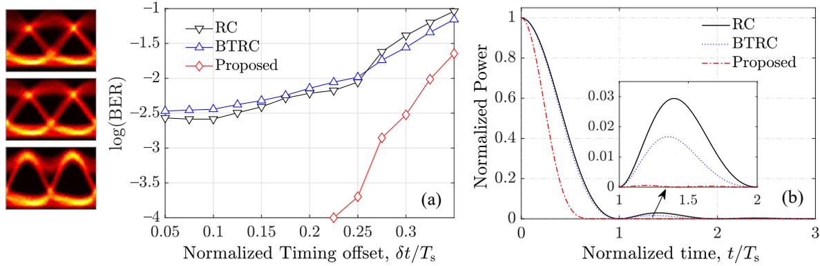
Fig. 2. (a) Bit error rate performance versus the normalized timing-offset of the received pulses at an emitted terahertz power of  $-13.3$  dBm. The eye diagrams are plotted for the RC, BTRC, and the proposed pulses from top to bottom, respectively, at a normalized timing-offset of 0.05. (b) The power profile of the three considered pulses. The roll-off factor is fixed at  $\alpha = 0.35$  for the RC and BTRC pulses, whereas, for the proposed pulse,  $\alpha = 0$  and  $\zeta = 10.47$ .
