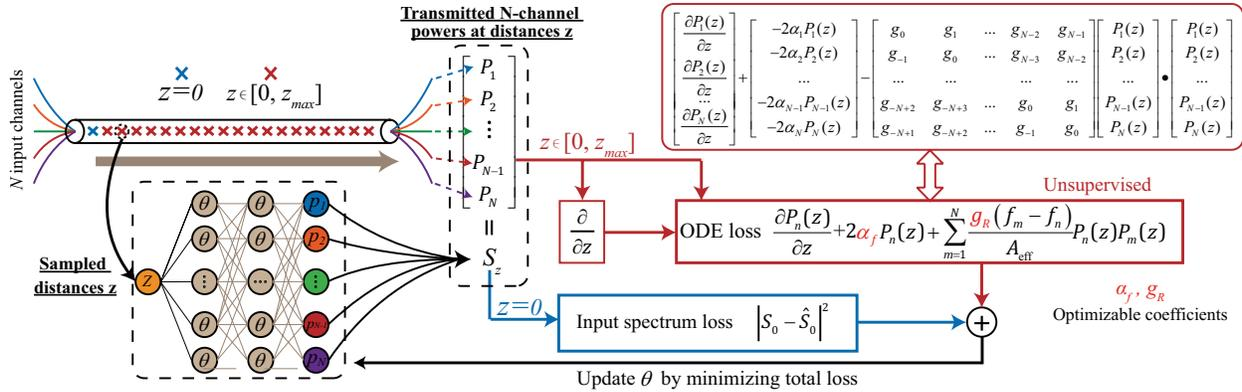
Fig. 1 Schematic of the PINN for multi-channel power evolution accounting for SRS. The ODE loss function is a matrix of the power evolution ODEs.  $\theta$  denote the parameters of NNs to be optimized.  $\hat{s}_0$  denotes the input power spectrum of fiber.
