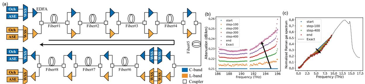
Fig. 2 (a) Experimental setup for C+L-band transmission. Process of characteristics identification for (b)  $\alpha_f$  and (c)  $g_R$  with respect to frequency.
