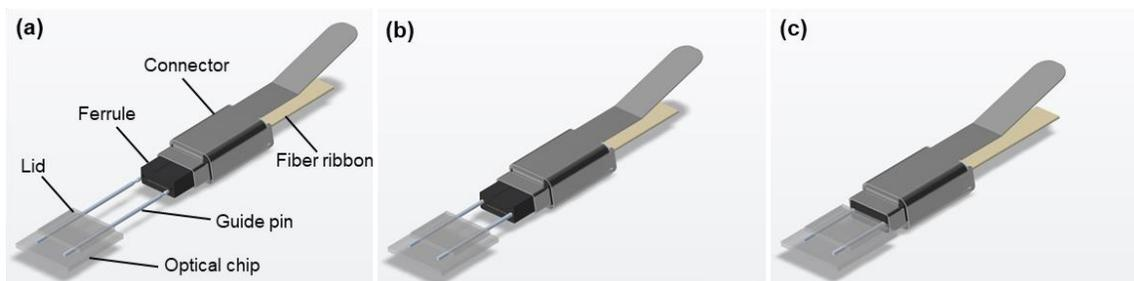
Fig. 1. Mating sequence to an optical chip in three steps: (a) guide pins engage with the ferrule, (b) guide pins sliding through the bores of the ferrule, and (c) connector completely mated with the optical chip.
