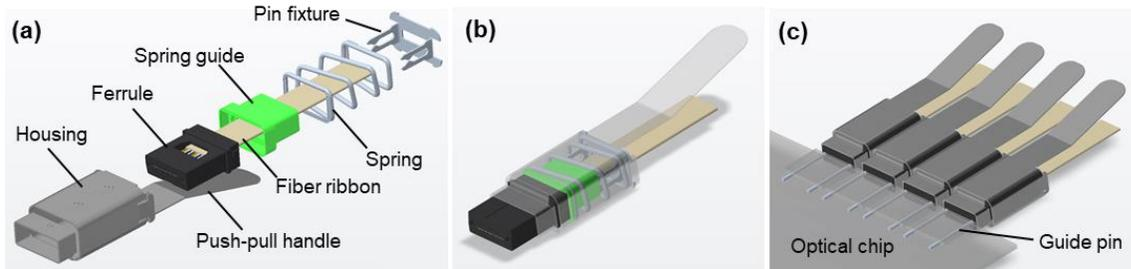
Fig. 2. 3D design view of the (a) exploded connector, (b) assembled connector, and (c) four mated connectors to on optical chip with eight assembled guide pins.
