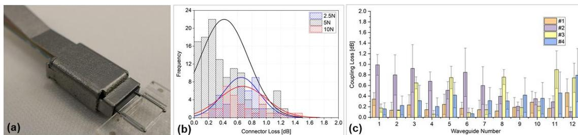
Fig. 4. (a) Mated connector with optical chip, (b) connector loss for random mating study for different connectors with 2.5 N, 5 N and 10 N spring force, (c) average coupling loss for 12 measured waveguides of four different optical chips (#1-4) with at least two mating cycles.
