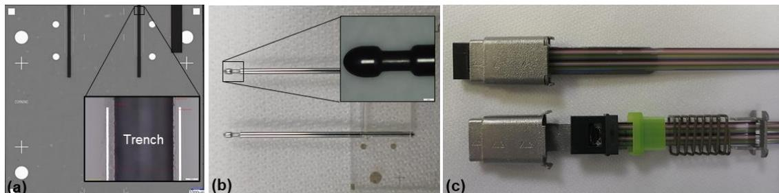
Fig. 3. (a) optical chip with a pair of trenches, (b) guide pins with trench assembled to the optical chip, (c) prototype of plug before and after assembly
