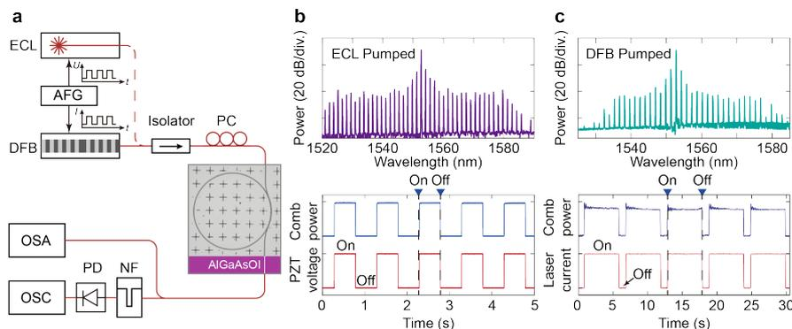
Fig. 1. (a) Experimental setup for the turnkey AlGaAs dark-pulse microcomb generation. (b) ECL and (c) DFB laser chip driven comb spectra and the comb power variations along with the control signal in five consecutive switching tests.
