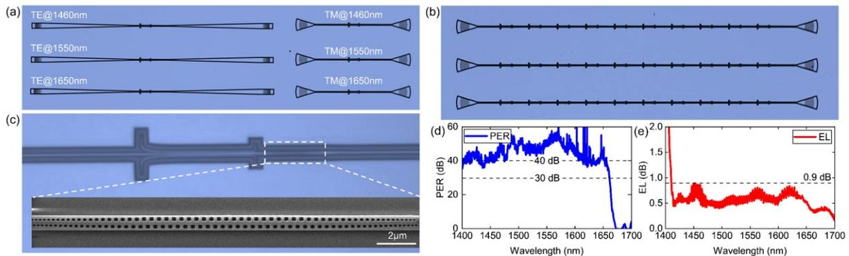
Fig. 3. (a) Microscopic image of fabricated three set devices for measurement. (b) Microscopic image of the 10 cascaded devices. (c) Microscopic image of fabricated device. Insets: partial SEM image of the Bragg grating. The measured PER (d) and EL (e) spectra for 1400-1700 nm.
