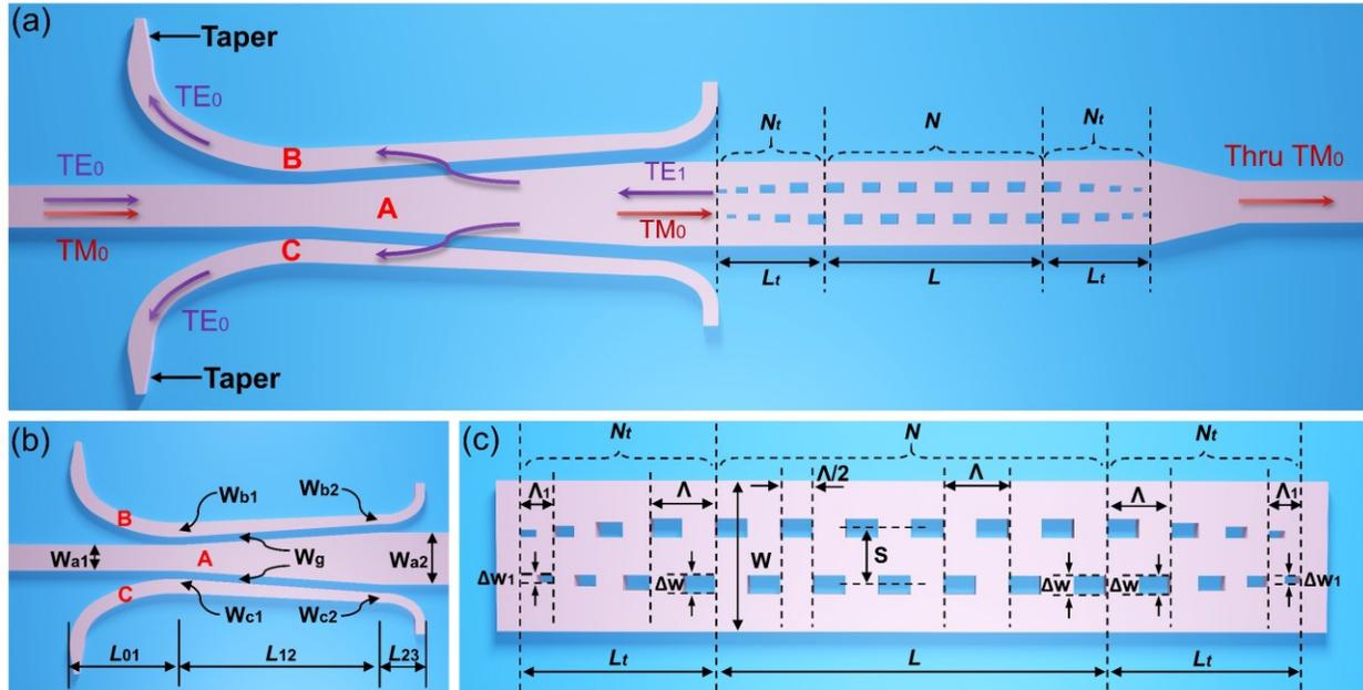
Fig. 1. (a) Top view of the proposed TM-pass polarizer based on MASABG. The black dashed lines show the three parts of MASABG: one uniform Bragg grating and two apodized Bragg gratings. The purple arrows show the propagation of the  $TE_0$  mode, and the red arrows represent the propagation of the  $TM_0$  mode. (b)  $TE_1$  mode filter based on a triple-core adiabatic taper. (c) MASABG with detailed parameters labeled.
