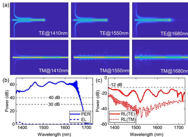
Fig. 2 (a) Calculated light propagation profiles when TE/TM polarization is launched. (b) Calculated PER and EL for the proposed TM polarizer at wavelengths range from 1400 to 1700 nm. (c) Calculated TE/TM reflections at wavelengths range from 1400 to 1700 nm.
